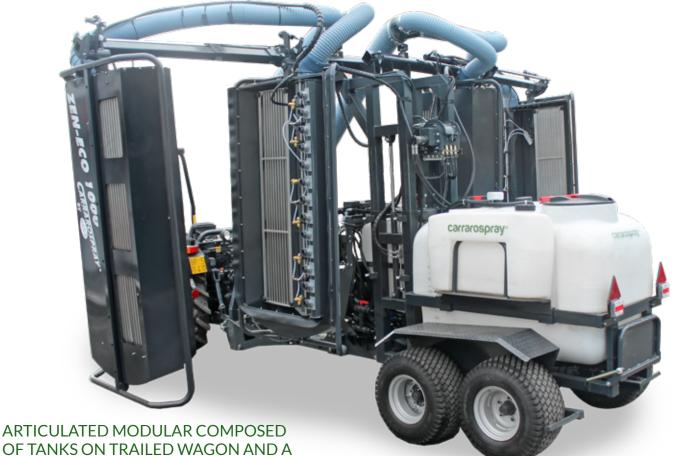
OF TANKS ON TRAILED WAGON AND A BLOWER MACHINERY ON LIFT OF THE TRACTOR
