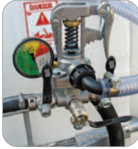
Pressure regulator valve at 3 ways 5-20 bar
