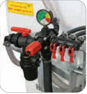
Pressure regulator valve at 3 ways 0-10 bar
