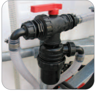
Suction filter with shut-off valve and 3 ways valve for quick washing circuit for chemical residus
