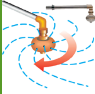
Jet for clean-washer inside the tank
